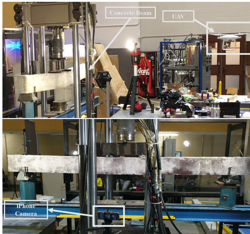
Figure 6. Experimental Setup showing (above) simply supported concrete beam transversely loaded at two points at its center and the video of the experiment being acquired using UAV, (below) and a still ground-based iPhone camera on a tripod is used to record the same experiment.
