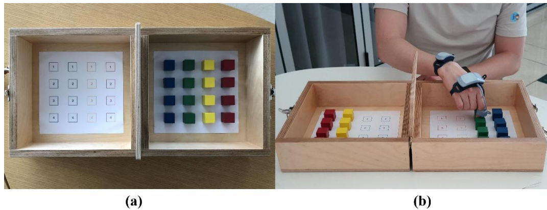
Figure 5. Experimental set-up: (a) configuration of the targeted box and block test and (b) positioning of the clip-on IMU-system to assess hand and wrist movements.
