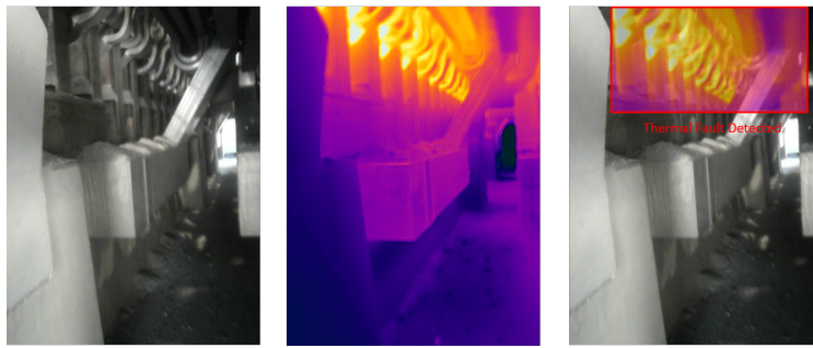
Figure 26. Thermal anomalies detection on-site for test run 4.
