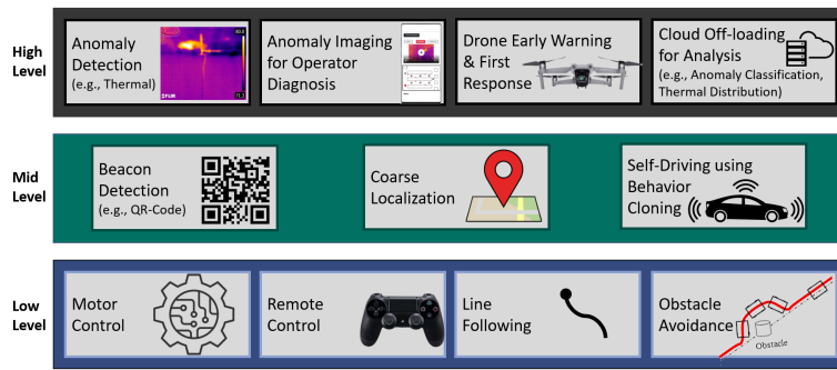
Figure 2. Robot surveyor operating system architecture with modular sub-systems. The architecture is general and adaptable to different applications through the high-level layer.
