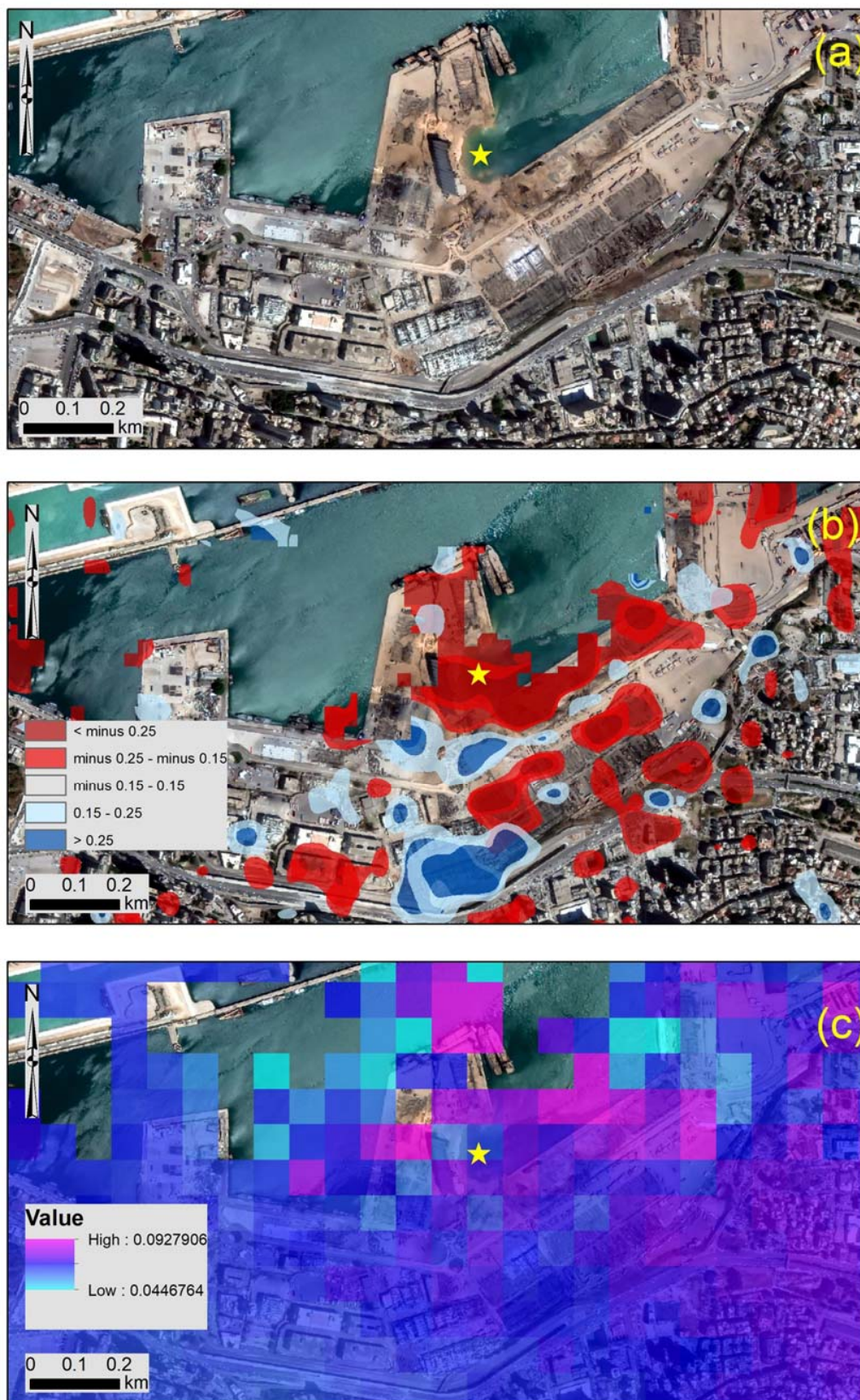
Figure 13. (a) High-resolution WorldView-2 image taken some hours after the explosion over the harbor of Beirut. The blast site is indicated with a yellow star. (b) Change detection as generated from the VV and VH log differences of the Sentinel-1 image and (c) the InSAR analysis (LOS of the descending orbit images) over the area. The location of the blast site is shown with the yellow star.
