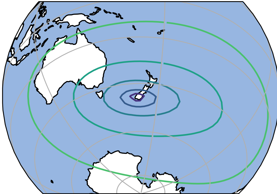
Figure 3. Global Doppler least-squares contours of L_{\nu} . This shows a global minimum close to the receiver position in New Zealand. This map is an orthographic projection of the globe, centered over New Zealand at longitude 170^{\circ} , and latitude 45^{\circ} south. The grey lines are 30^{\circ} intervals in longitude and latitude.
