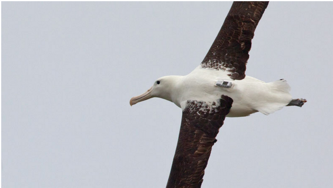
Figure 8. A solar-powered FastFix tag attached to the back of a Royal Albatross. This tag can store in a 2 GB SD-card approximately a quarter of a million fixes. Photo ©Keith Payne—used with permission.
