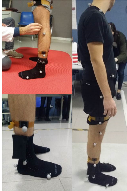
Figure 5. Subject equipped with both systems: SWEET Sock and reflective markers.
