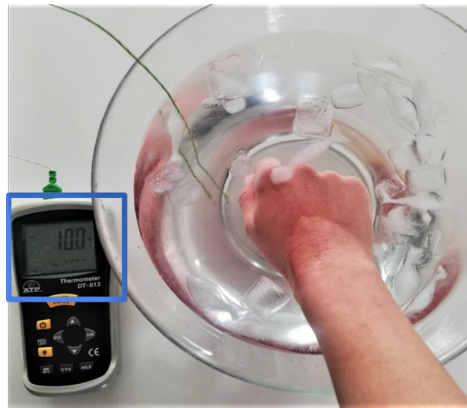
Figure 8. The set-up for the thermal protocol using hand immersion in iced-cold water at 10 °C.
