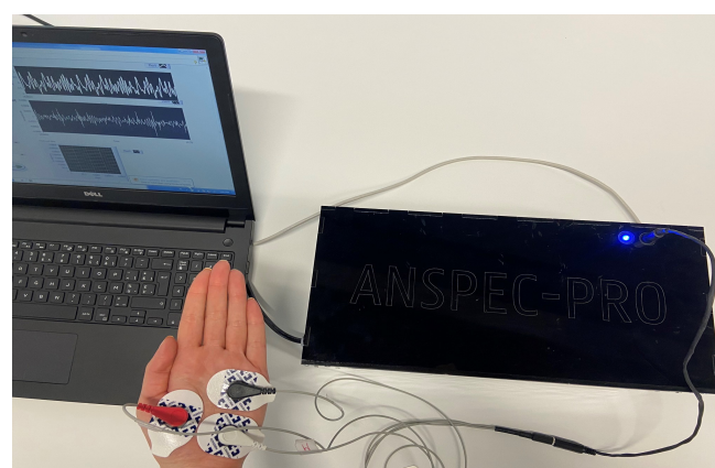
Figure 1. The second generation ANSPEC-PRO prototype and related set-up for non-invasive measurement of skin impedance.
