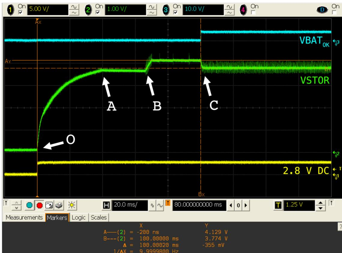
Figure 5. Behavior of BQ25504 when a partially charged battery is attached.
