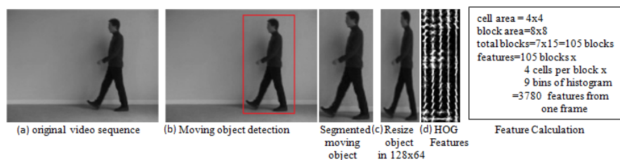
Figure 4. Proposed feature extraction technique: (a) Original video sequence. (b) Detected moving object. (c) Resize detected moving object into 128 \times 64 size. (d) Histogram oriented gradient (HOG) feature extraction.
