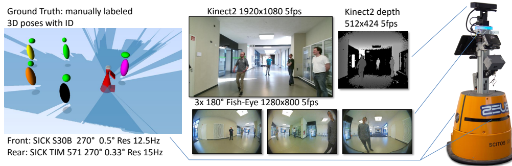
Figure 5. Dataset used for evaluation and the robot which has been used for recording (published in [22]) The sensor equipment for recording the dataset was similar that of the robot used in the real training application (see Figure 1) except the mounting point of the Kinect2 RGB-D camera.
