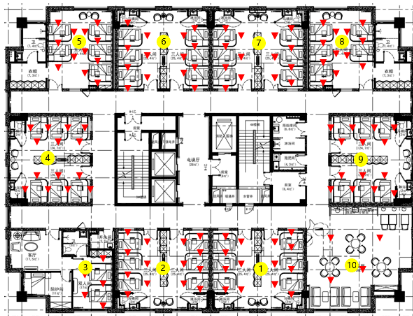
Figure 6. The schematic diagram of the test environment, where the rooms and RPs are labeled with yellow circles and red triangles, respectively.
