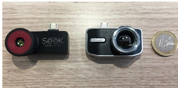
**Figure 1.** Selected thermal cameras: ST (left) and TE-Q1 (right).
