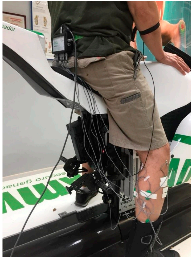
Figure 1. Right EMG electrodes positioning and their channels (E1–E7).
