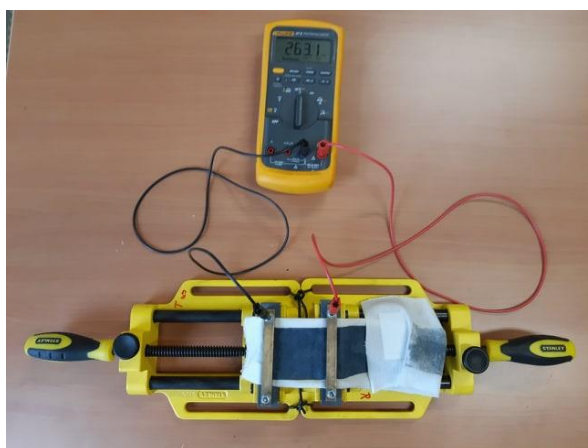
Figure 5. Two-point method resistance measurements set-up.
