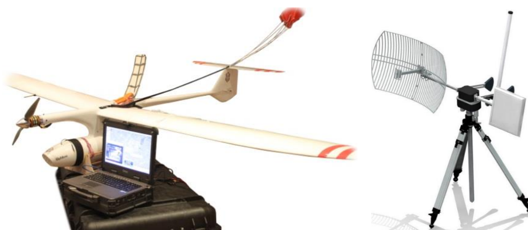
Figure 2. Unmanned aerial system (UAS) components: mini-UAV with the video head and recovery parachute, portable Ground Control Station—transported in a container, communication terminal.
