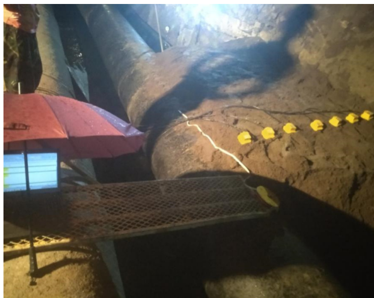
Figure 4. Photograph showing the measurement arrangement for ground surface vibration.
