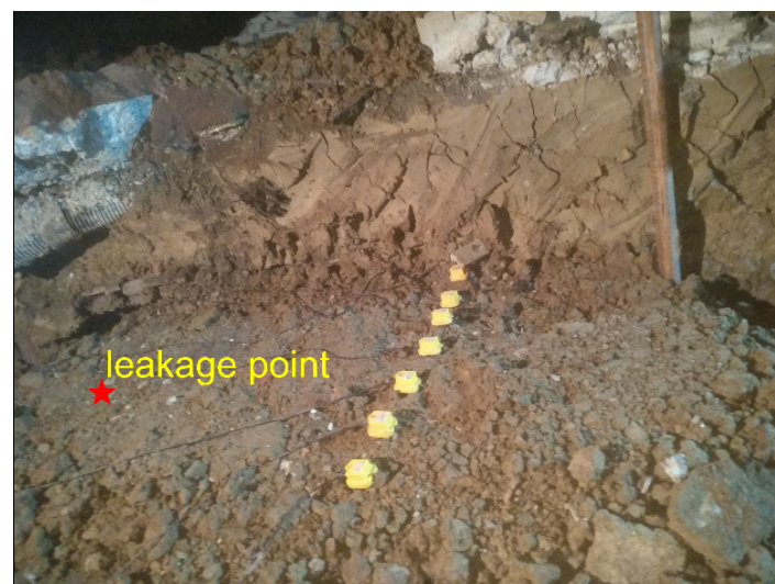
Figure 6. Ground surface vibration measurement using the sensor array at the distance of 1 m from the leak.
