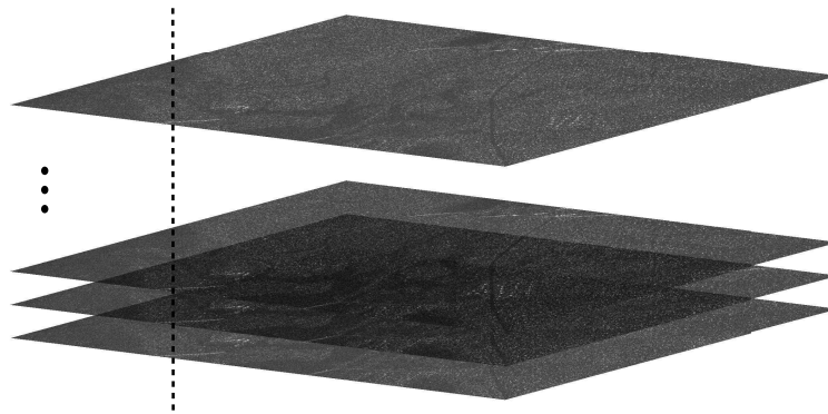
Figure 2. Stack of images to be considered in GSP. The methods should be applied for each pixel position, as evidenced by the vertical line.
