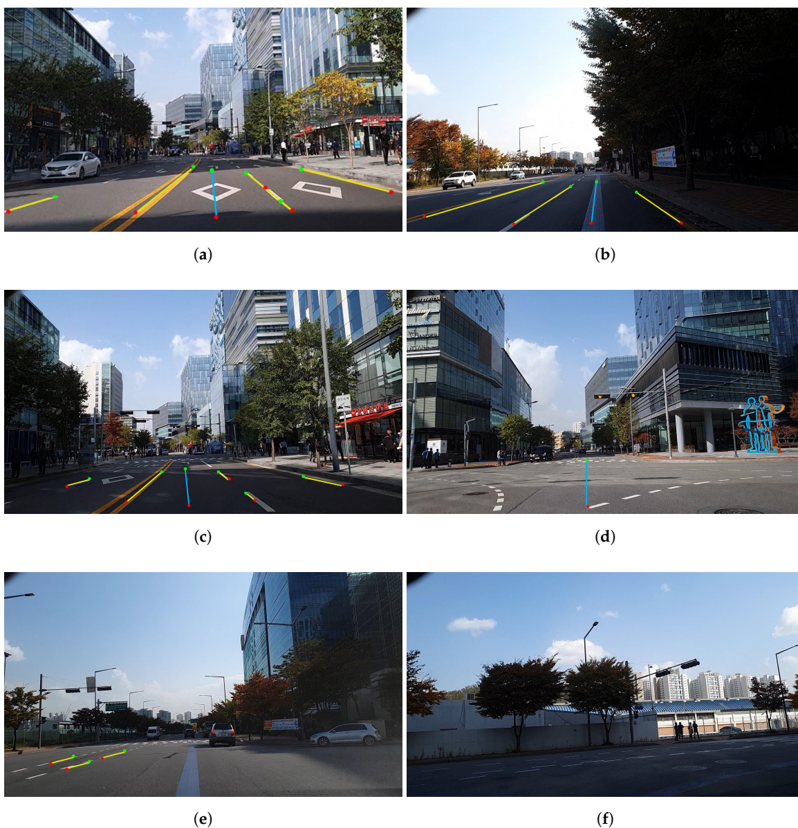
Figure 11. Results of driving link extraction in course 2: (a,b) correct detection of vehicle lines and extraction of driving link in the changes of illumination; (c) correct extraction of driving link by detecting yellow lane marking; (d) update previous driving link; (e,f) extraction failure.
