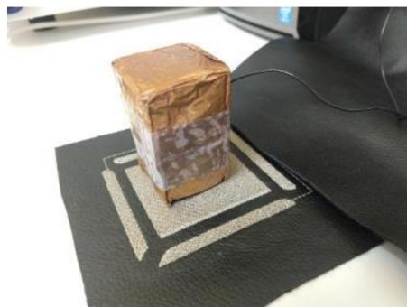
**Figure 7.** “Artificial hand” provided by Microchip made of Styrofoam covered by copper and connected to ground.
