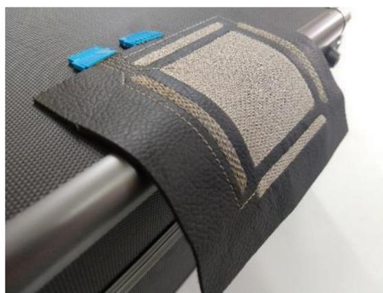
**Figure 9.** Flexible 3D Boosted sensor manufactured.
