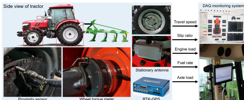
Figure 4. Configuration of load measurement part of the agricultural field measuring system.
