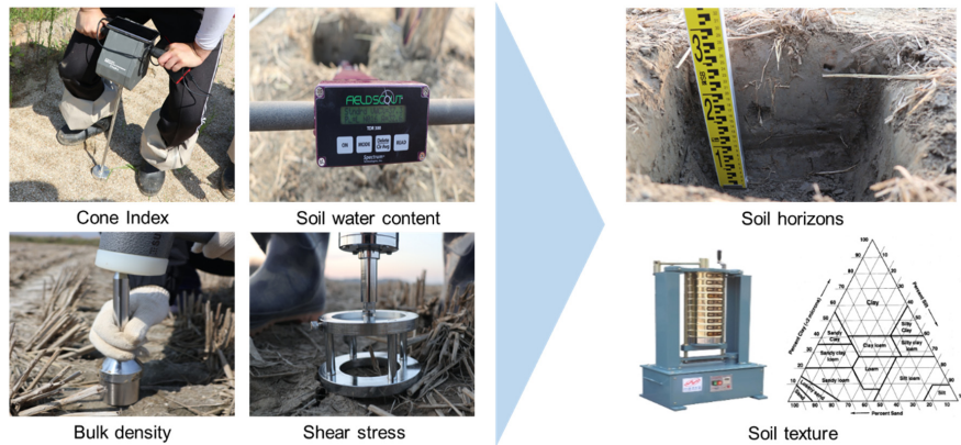
Figure 2. Overall test procedure of the soil property measurement.
