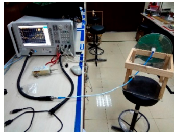
Figure 23. Photo of the VSWR measurement setup using the N5227A PNA Microwave Network Analyzer.
