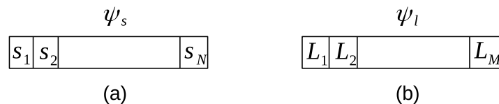
Figure 2. Illustration of the time-based windows. The sensor time-based window is of length \psi_s , and the time duration is computed for each sensor. The location time-based window is of length \psi_l , and the time duration is computed for each location: (a) sensor time-based window; (b) location time-based window.
