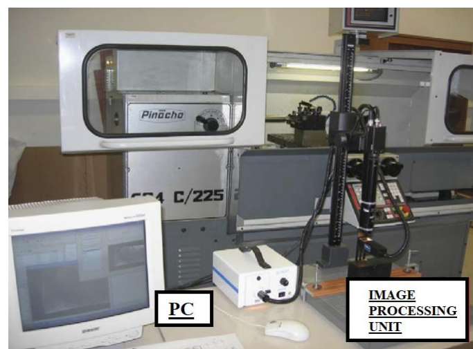
Figure 10. An example for image processing based tool condition monitoring system [77].
