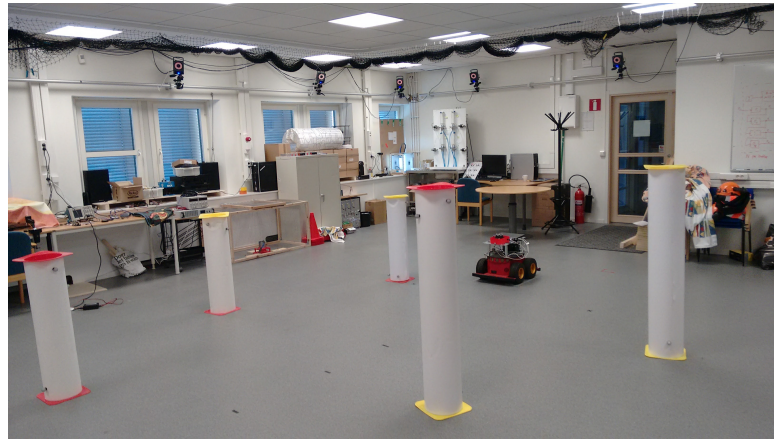
Figure 3. Setup of a typical calibration experiment, comprising five landmarks (white cylinders) and the robot–sensor system of Figure 4 moving among the landmarks.
