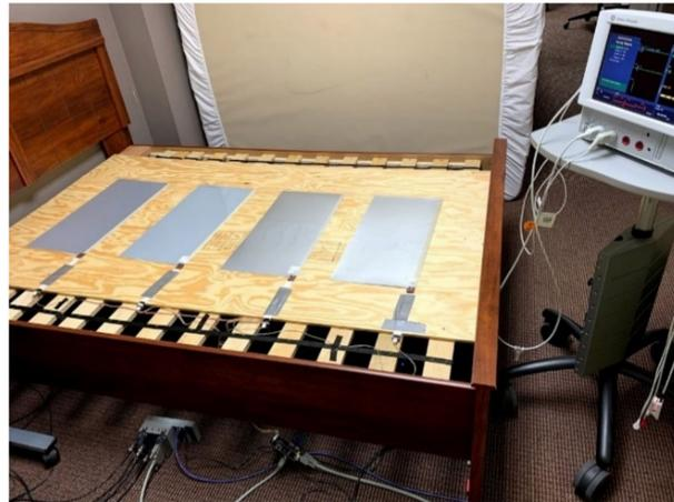
**Figure 3.** Image of the bed system from another angle, accompanied by the CardioCap 5 patient monitor. The analog conditioning and National Instruments data collection hardware can be seen under the bed.
