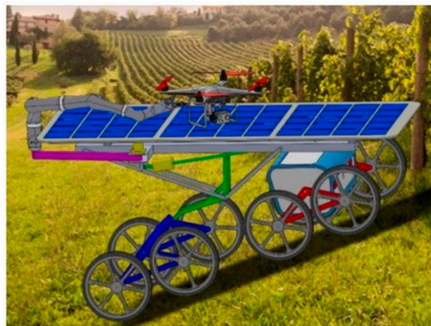
Figure 12. UGV-unmanned aerial vehicle (UAV) cooperative concept [176]. (CC BY 4.0).
