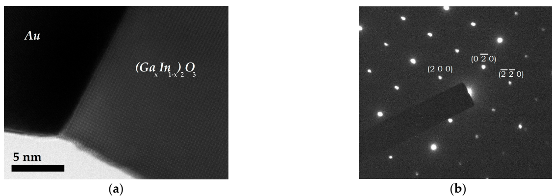
Figure 5. (a) High resolution TEM image of the interface between NW of the Sample A and its gold tip and (b) the corresponding diffraction pattern of the NW, with some of its peaks indexed. The diffraction pattern is coherent with cubic \text{In}_2\text{O}_3 , observed along its zone axis [001].
