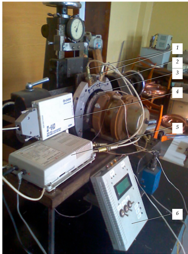
1—Single-coil eddy current sensors; 2—Stator; 3—Protrusion of the measuring disk; 4—Module E14-440 by L-Card; 5—Block of measuring transducers; 6—Signal processing unit
