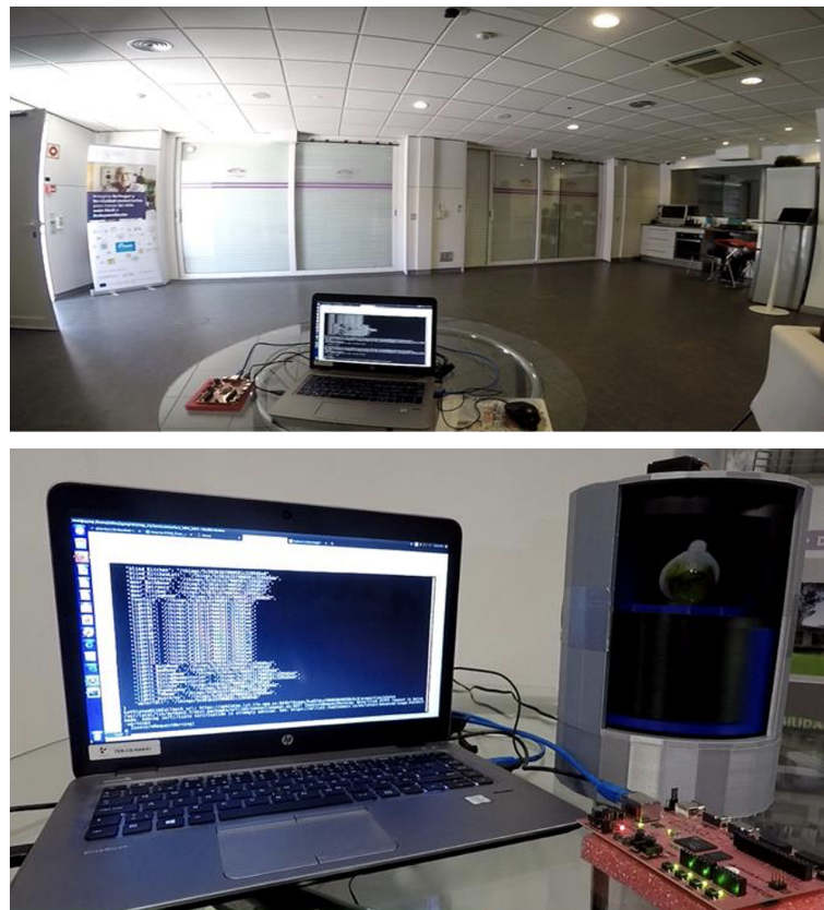
Figure 11. Field Programmable Gate Array controlling KNX ® devices (upper image) and an IoT device (lower image) via LLG.
