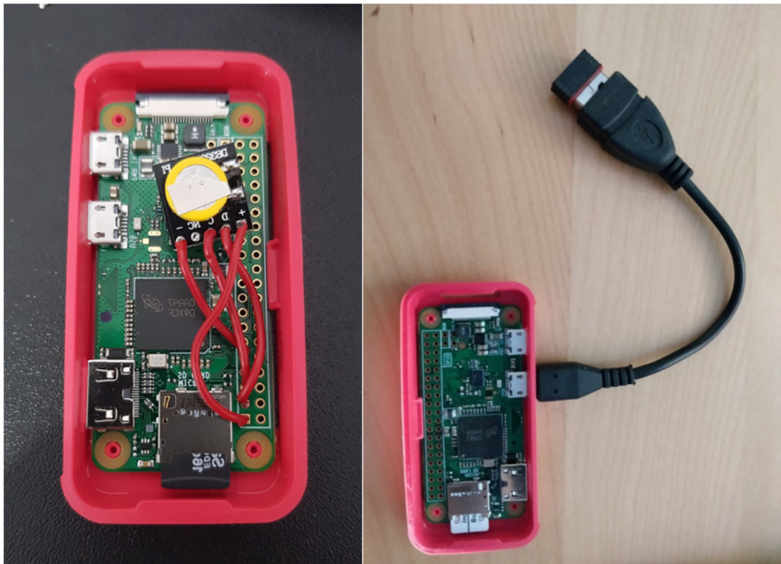
Figure 4. Wi-Fi sensor prototype showing the RTC clock (left) and the external Wi-Fi adapter (right).
