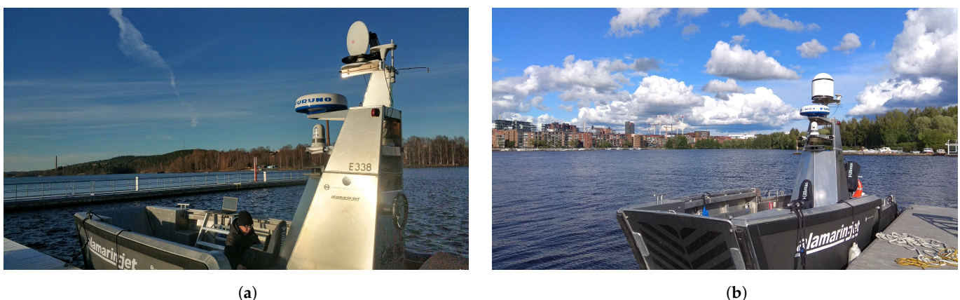
Figure 11. Photo of the USV with installed communication equipment. (a) Final implementation of the USV without the dome on the directional antenna; (b) Final implementation of the USV with the dome on the directional antenna.
