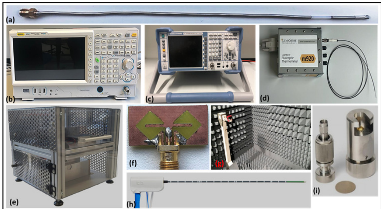
Figure 2. MWA experimental setup: (a) self-developed microwave applicator with a single slot; (b) spectrum analyzer; (c) VNA ; (d) LumaSense temperature probe; (e) high-power RF source; (f) BMA; (g) anechoic chamber; (h) Covidien Emprint™ Standard Percutaneous Antenna with Thermosphere™ Technology; (i) N1501A high-temperature probe kit.
