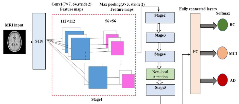
**Figure 5.** The framework of the proposed method.
