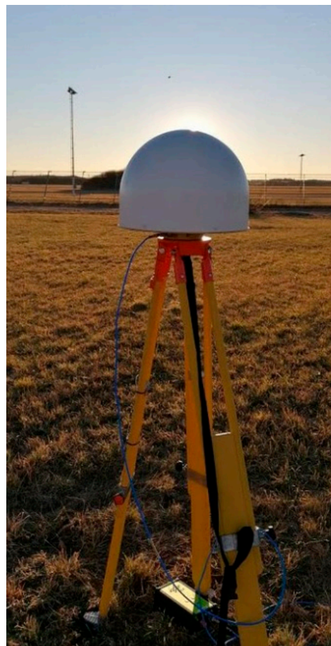
Figure 9. Leica AR25R4 antenna placed on a tripod in DLR campus field for GNSS measurement.
