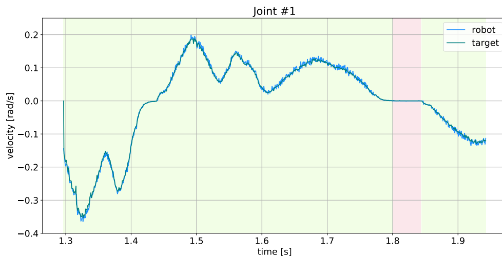
(b) The actual velocity of the robot and the set (target) speed.
