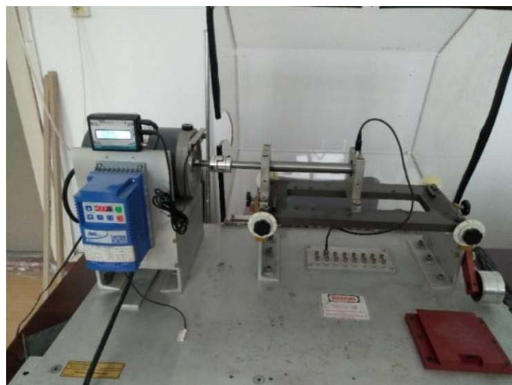
Figure 6. Test rig used to collect different speeds and different sample rate data.
