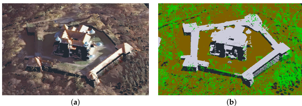
Figure 13. ISOK point cloud: scanning colors (a); class colors (b).
