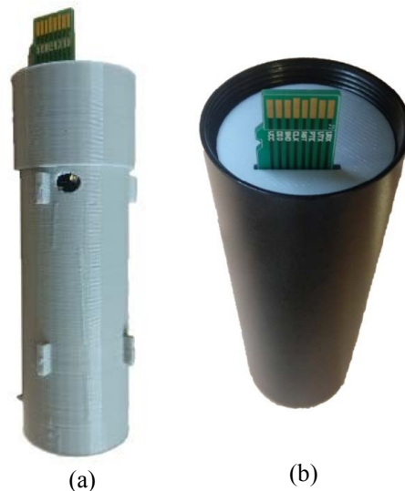
Figure 11. Underwater sensor node construction details: (a) PLA holder for node capsule with the main board and battery, and (b) holder inside of the container.
