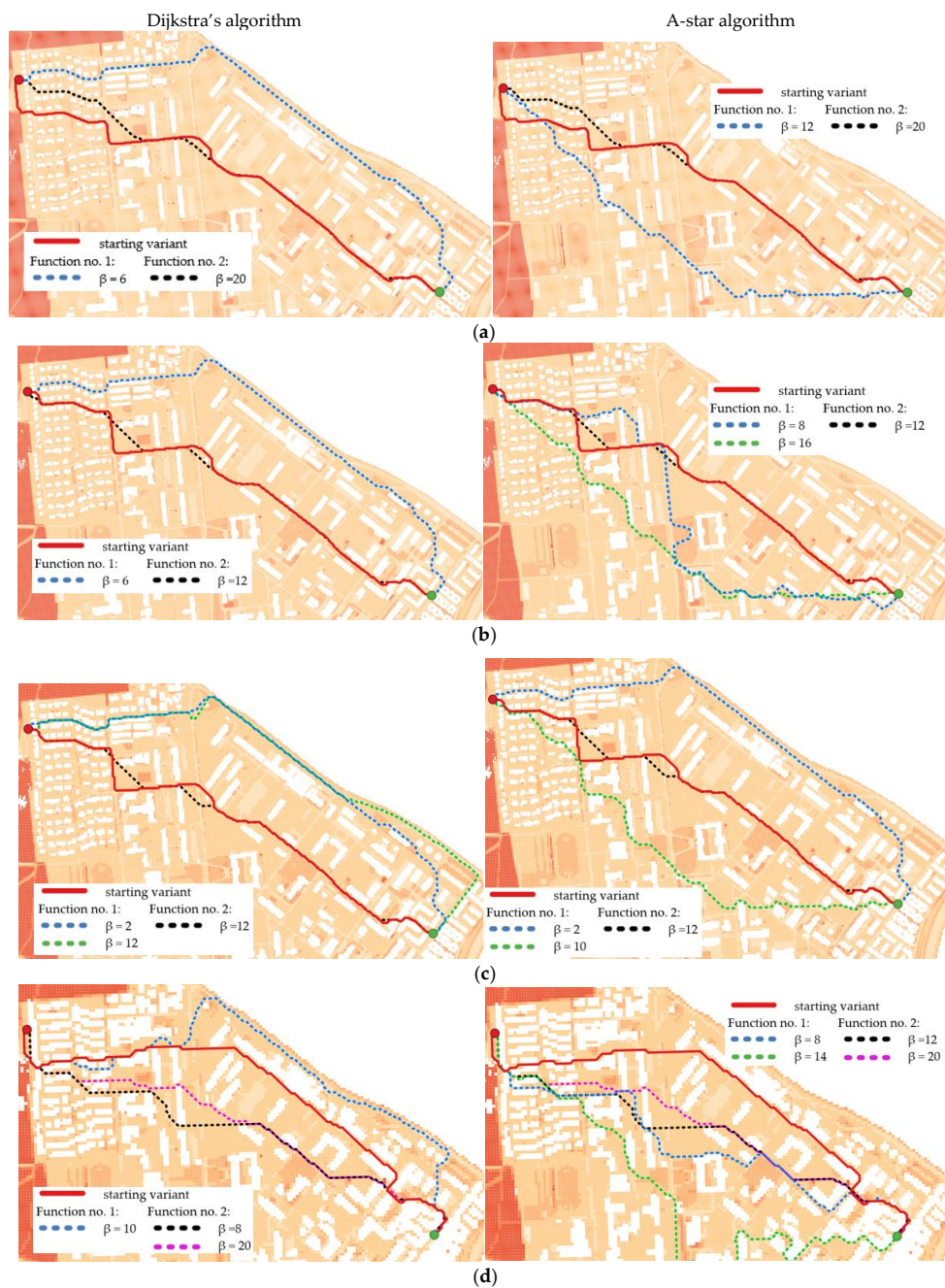
Figure 13. Optimal routes in urban area in different configurations and in the following resolutions: (a) 2 m; (b) 3 m; (c) 5 m; (d) 10 m.
