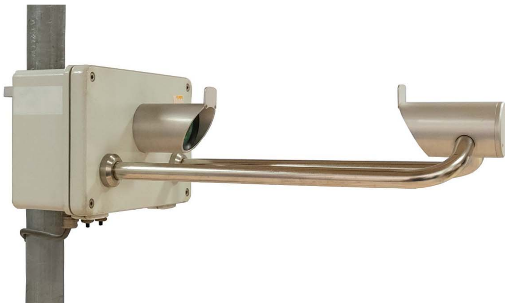
Figure 1. The Thies LPM [25], with the emitting head (attached to the circuitry box on the left-hand side) and the receiving head (attached to the supporting arms on the right-hand side).
