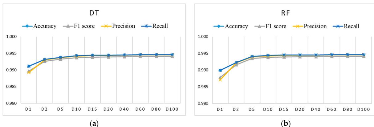
Figure 7. Evaluation results for imbalanced training datasets D_i using: (a) DT (coincidence of accuracy, recall, and precision only for datasets larger than D_1 ); (b) RF (coincidence of accuracy, recall, and precision only for datasets larger than D_1 ).
