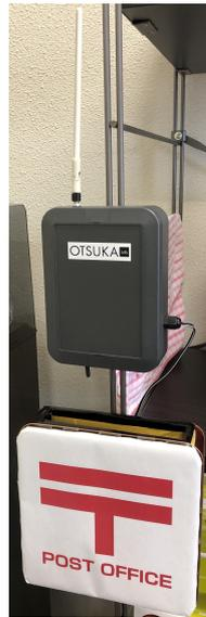
**Figure 6.** Prototype of Postbox 2 for the Kanbans.
