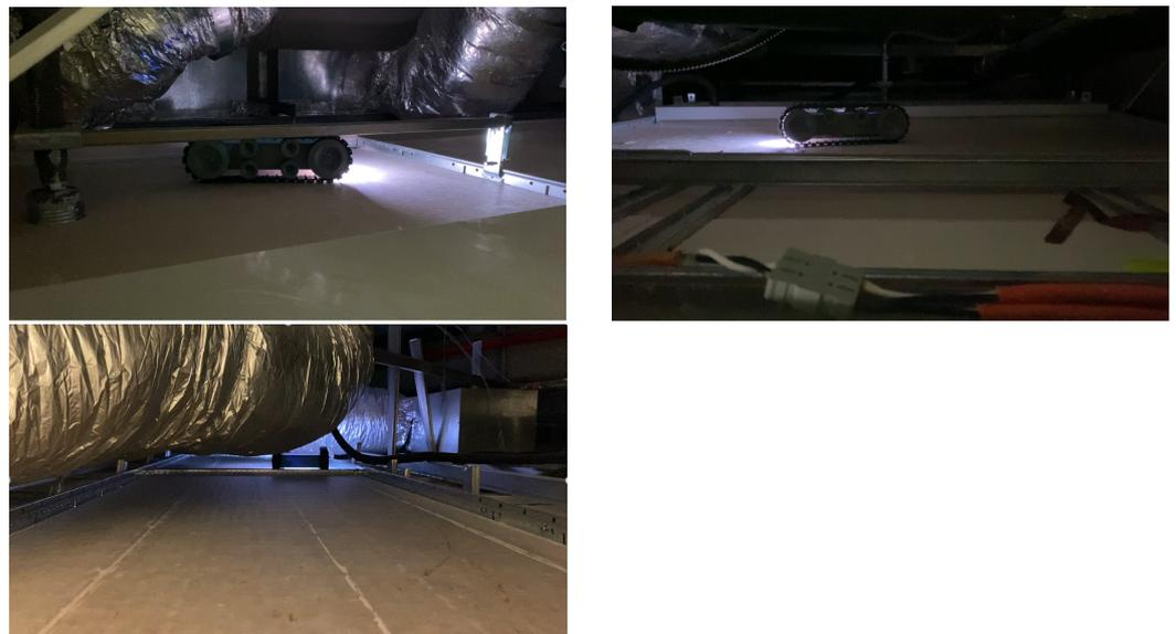
Figure 8. Falcon rodent activity inspection in a false ceiling environment.
