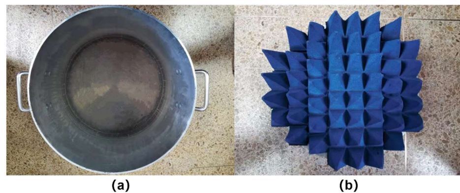
Figure 5. The physical picture of the calibration source. (a) Metal aluminum barrel; (b) Microwave absorbing material.
