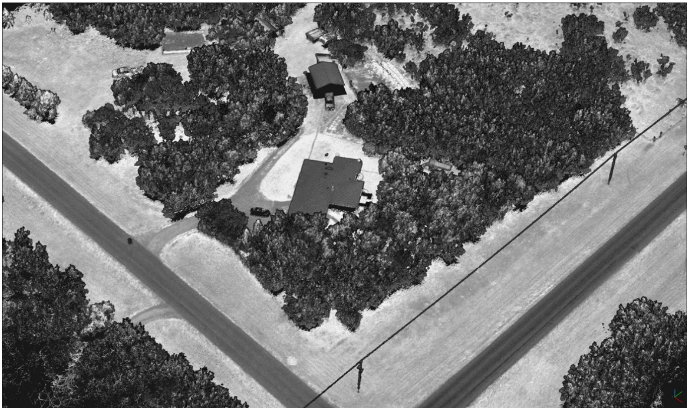
Figure 13. North–west looking-perspective view of the point cloud for flight A, colored by gray-scale intensity values.
