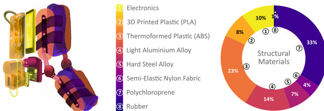
Figure 4. Materials used in the prototype and their percentage, proportional to the total volume.
