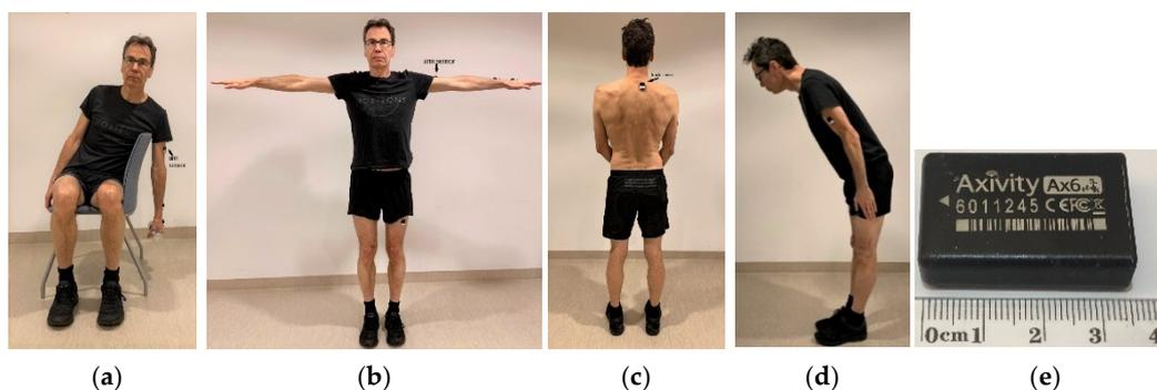
**Figure 2.** Calibration procedures for the arm and the trunk showing (a) the reference posture for the arm, (b) the posture for determining the direction of the sensor on the arm, (c) the reference posture for the trunk, (d) the posture for determining the direction of the sensor on the trunk, and (e) the AX6 inertial measurement unit.
