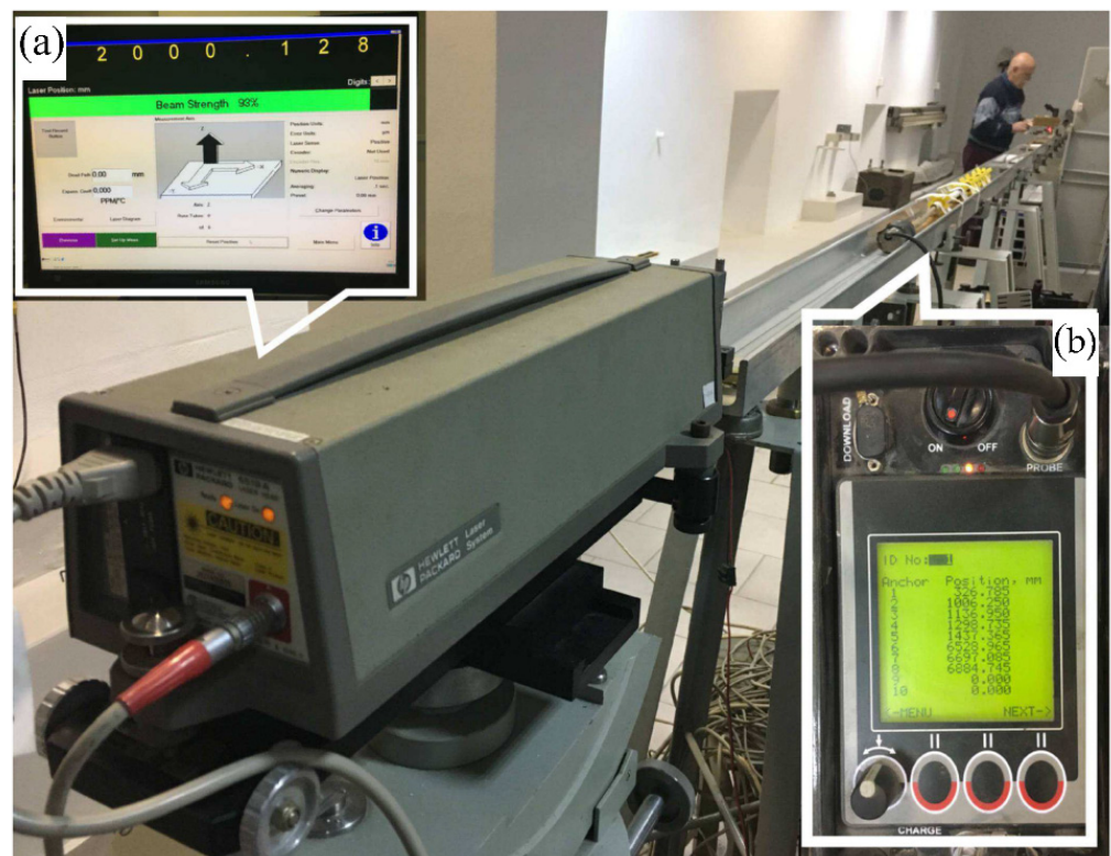
Figure 6. The UST AGH Surveying Comparator Laboratory. The laboratory tests measurements: using the HP interferometer: (a) the read-out device of the interferometer, (b) the read-out device of the extensometer.
