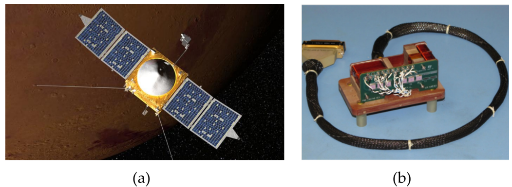
Figure 1. (a) Illustration of the Mars Atmosphere and Volatile Evolution (MAVEN) spacecraft in orbit over Mars. The magnetometer “boomlets” are located at both ends of the solar array panels. (b) MAVEN magnetometer sensor assembly [25]. Reproduced with permission from NASA/Goddard Space Flight Center.
