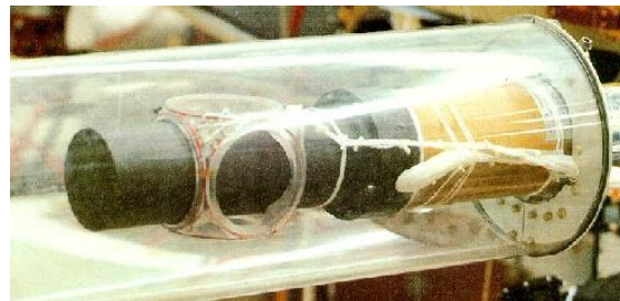
Figure 3. The Ulysses (1990–ongoing) Magnetic Field Investigation vector helium magnetometer (VHM) [39]. The flight model VHM used for the Cassini mission was originally developed as a backup for Ulysses, with later modifications added for operating range adjustment and to compensate for differing boom lengths [8]. Reproduced with permission from the European Space Agency.
