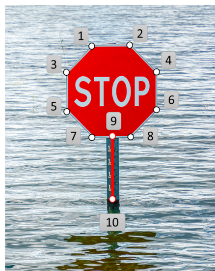
Figure 6. Illustration of the manual retrieval method. The points (1–10) indicate the critical edge for the sign shape and are used for dimension calculation.
